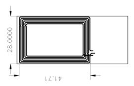
Antenna transmission frequency: 13.56MHz
