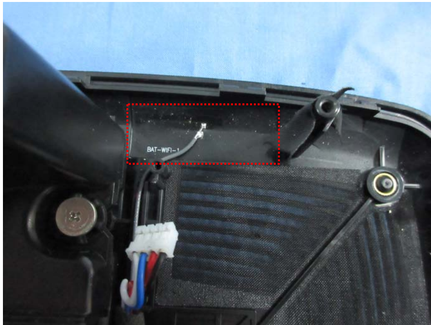
WiFi Antenna 1 View
