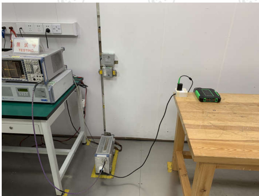
Conducted Emissions Test Setup
