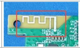
The antenna is PCB antenna.
