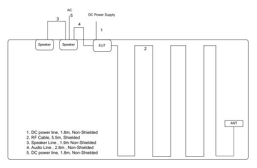
Test Configurations: 88~108MHz
