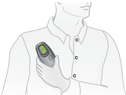
Figure 12. Correct positioning of sleep remote over generator
