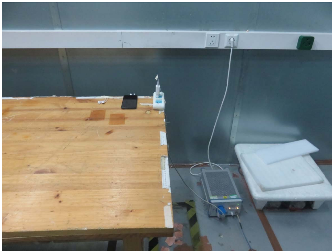
Picture 2 Conducted Emission Test Setup
