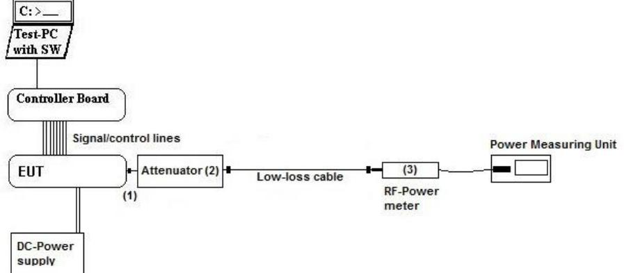
**Testing method:** ANSI C63.10:2013, KDB 558074 D01 DTS Meas.Guidance v03r05
