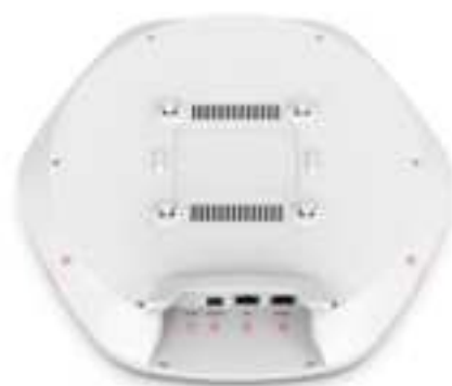
Figure 1-3 Physical interfaces of HS_C09961
