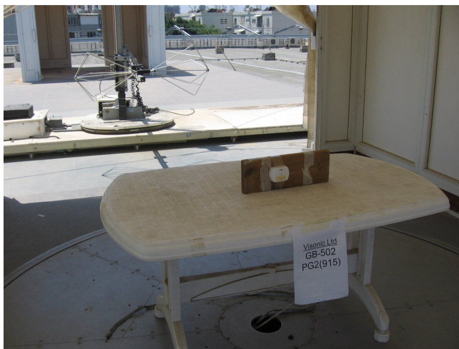
Figure 7. Radiated Emission Test – Wall Mounted
