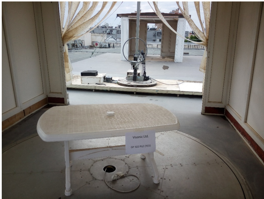
Figure 2. Radiated Emission Test – Ceiling Mounted
