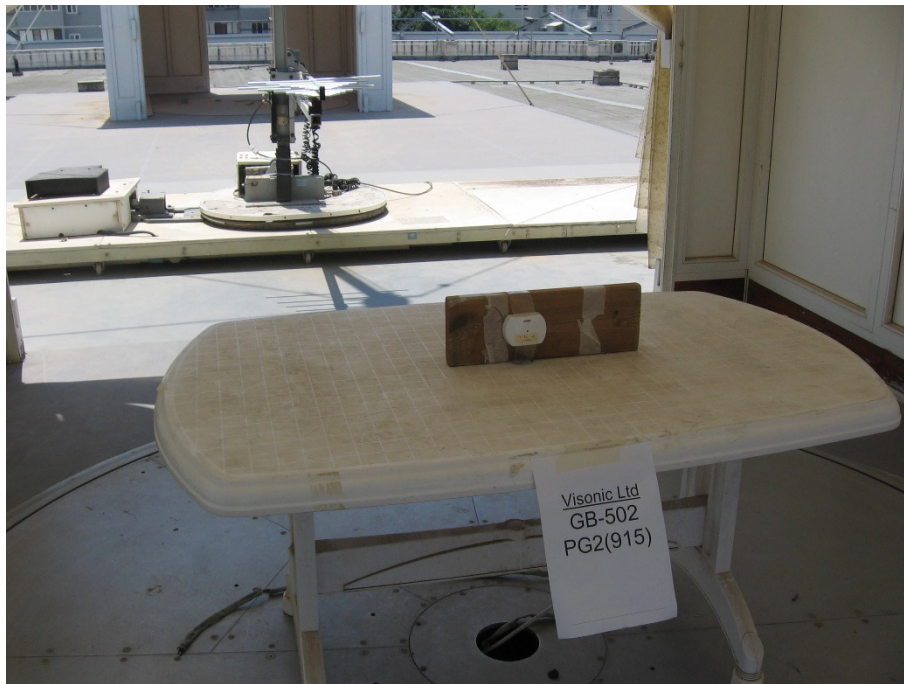
Figure 6. Radiated Emission Test – Wall Mounted
