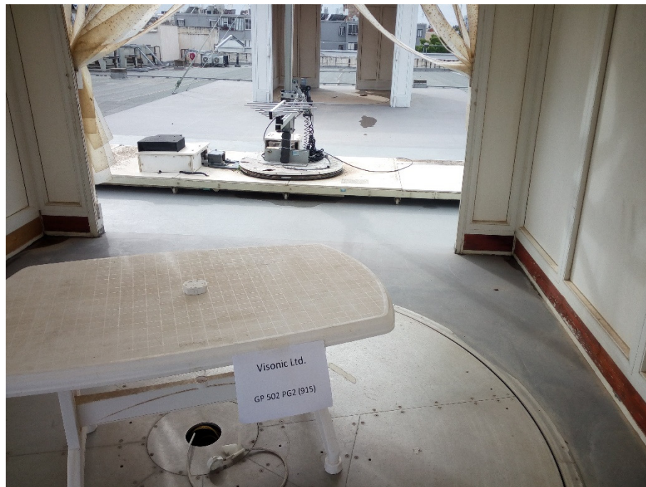
Figure 4. Radiated Emission Test – Ceiling Mounted
