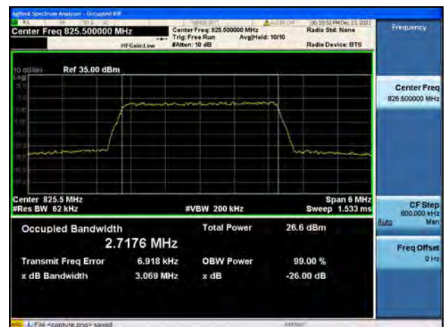
Band5 / 3MHz / Low CH / 64QAM
