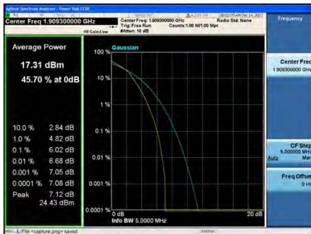
Band2 / 3MHz / Low CH / 16QAM
