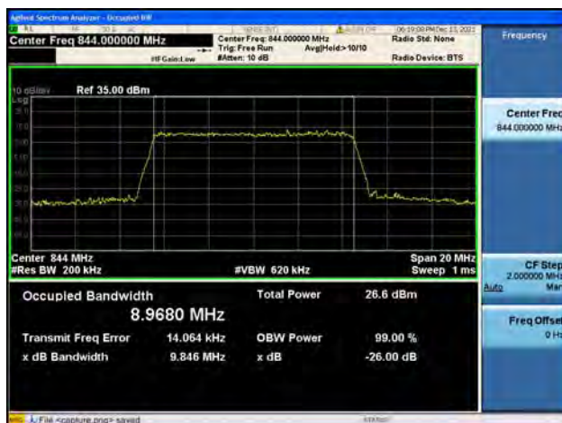
Band5 / 10MHz / High CH / 16QAM
