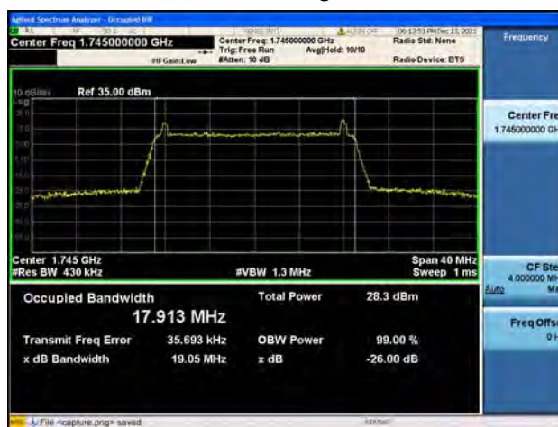
Band4 / 20MHz / High CH / 64QAM
