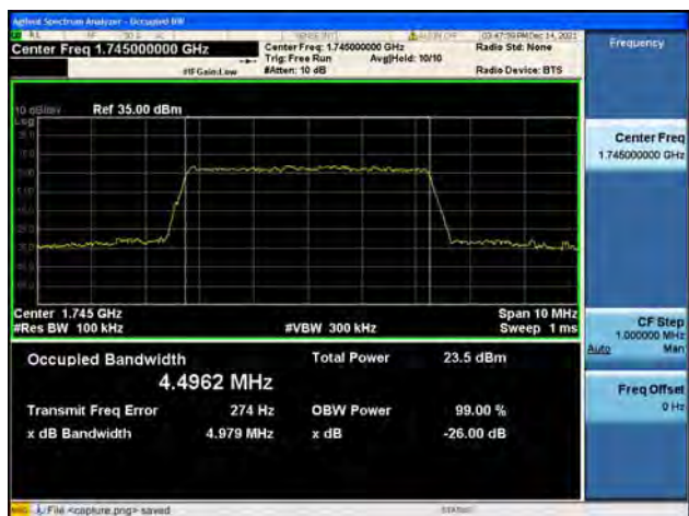
Band66 / 5MHz / Mid CH / 16QAM
