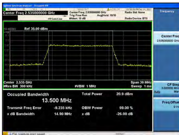
Band7 / 15MHz / Mid CH / 16QAM
