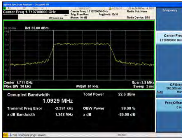
Band66 / 1.4MHz / Low CH / 64QAM
