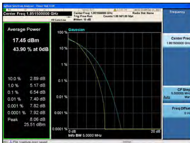
Band2 / 3MHz / Low CH / 16QAM
