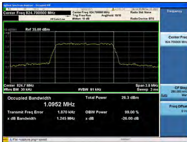
Band5 / 1.4MHz / Mid CH / 16QAM
