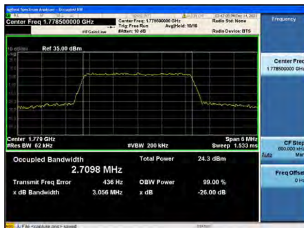
Band66 / 3MHz / High CH / 16QAM
