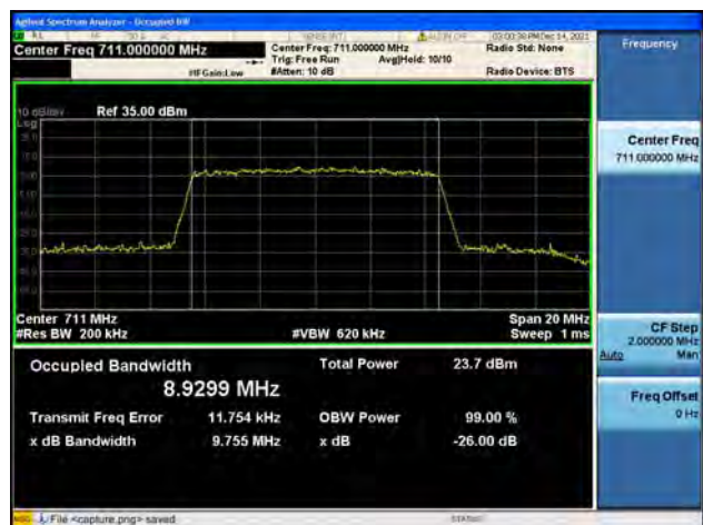
Band17 / 10MHz / High CH / 16QAM
