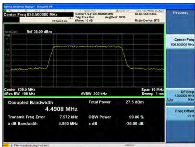
Band5 / 5MHz / Mid CH / 64QAM
