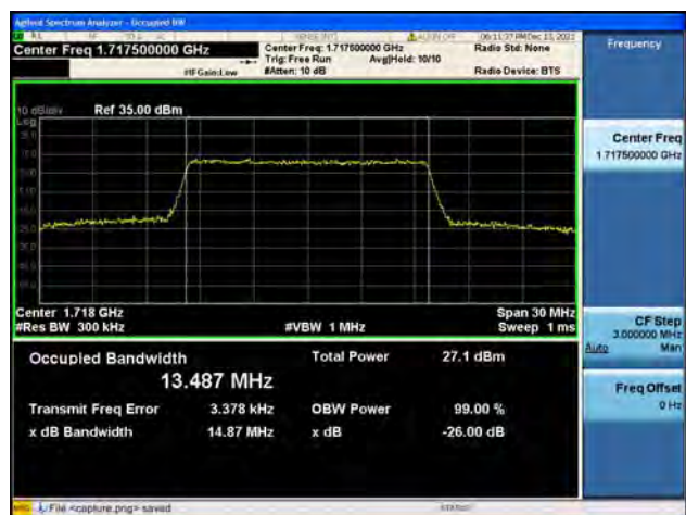
Band4 / 15MHz / Low CH / 64QAM
