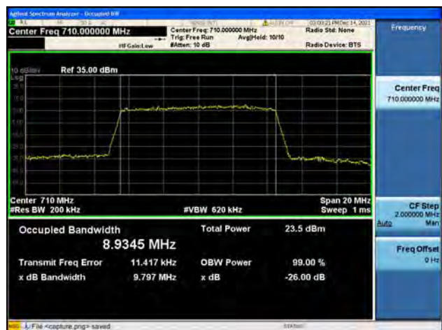
Band17 / 10MHz / High CH / 16QAM
