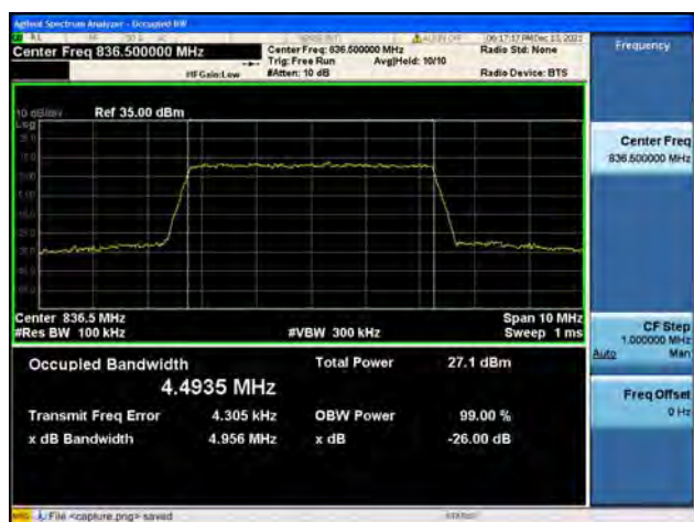
Band5 / 5MHz / Mid CH / 64QAM
