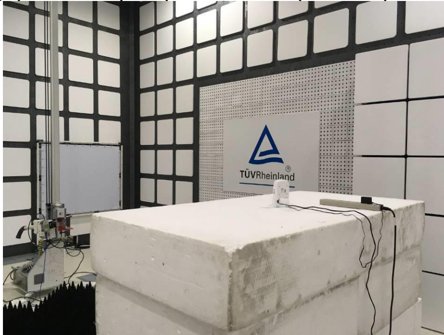
Photograph 6: Test Setup for Spurious Emissions (Back View 4)
