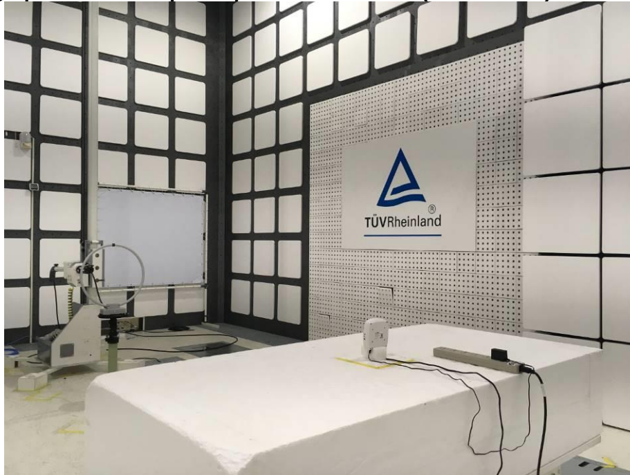
Photograph 4: Test Setup for Spurious Emissions (Back View 2)
