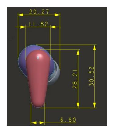
Note: The size of earphone is 28.21mm (L) \* 6.6mm (W). The space is not enough for FCC ID. Therefore, the FCC ID is shown in the UM.
