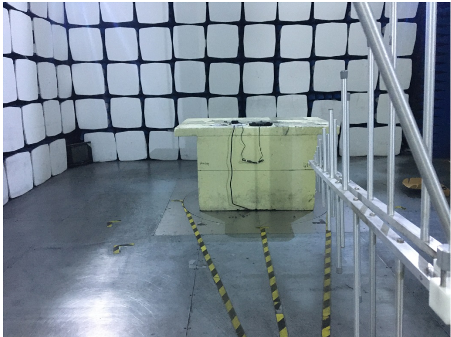
Radiation Emission Test Setup (30MHz to 1GHz)
