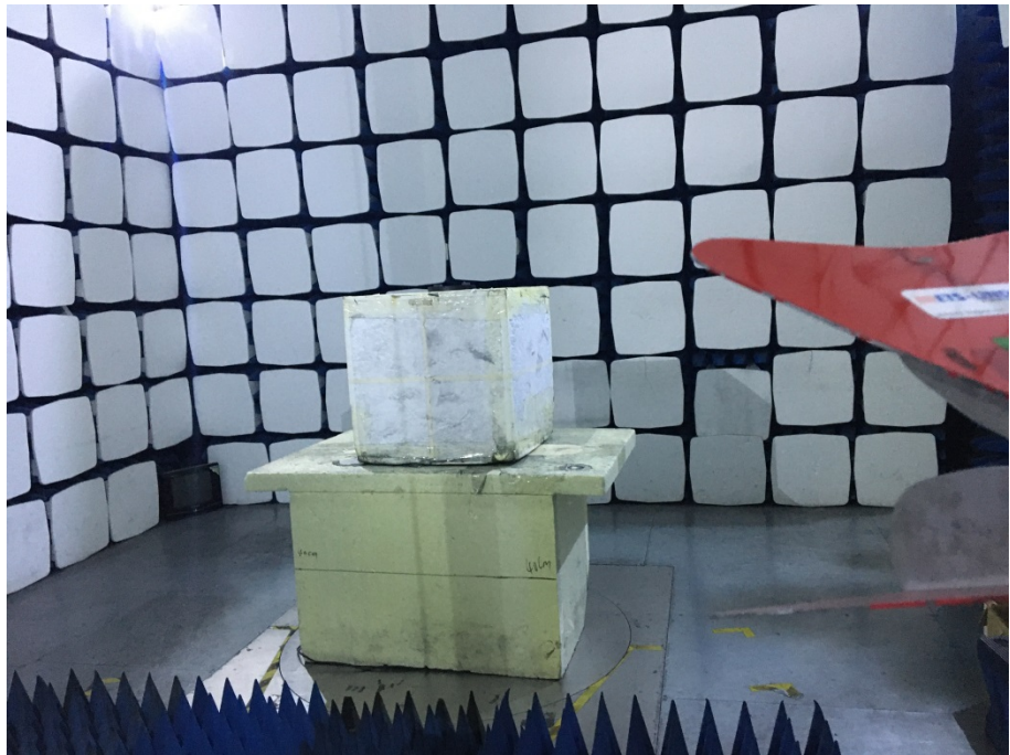
Radiation Emission Test Setup (1GHz to 18GHz)
