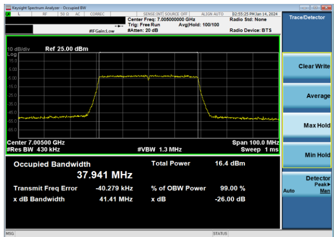
Plot 7-158. 26dB & 99% Bandwidth Plot Antenna 2a (40MHz 802.11ax (UNII Band 8) – Ch. 211, MCS4)
