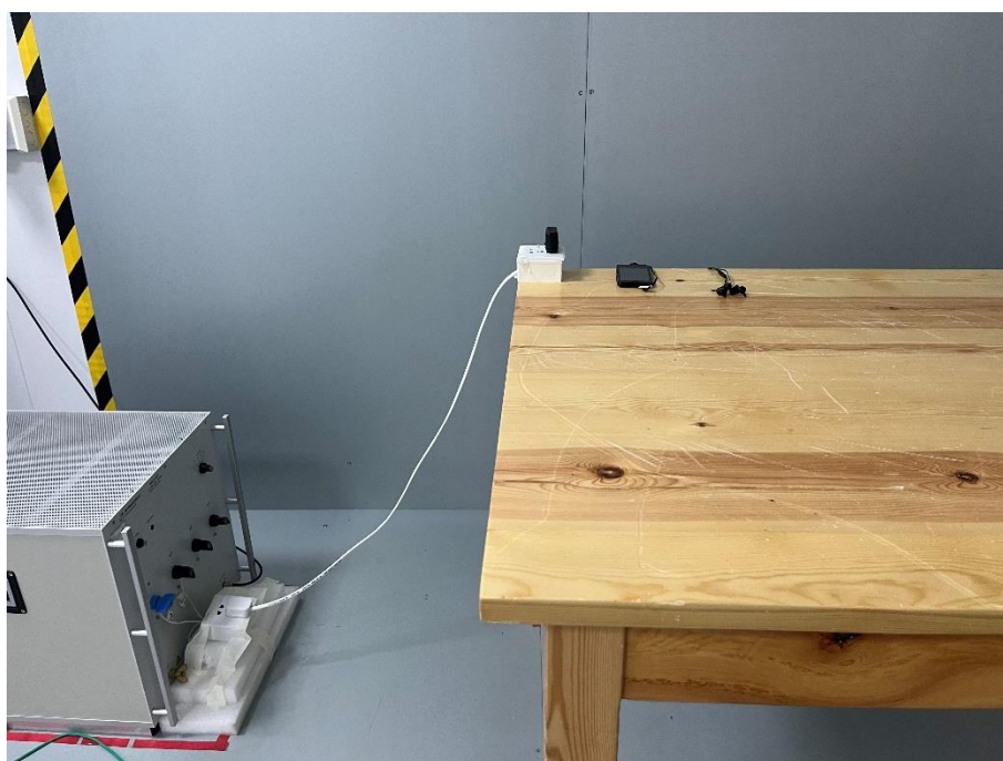
Conducted Emission Test Setup Photo
