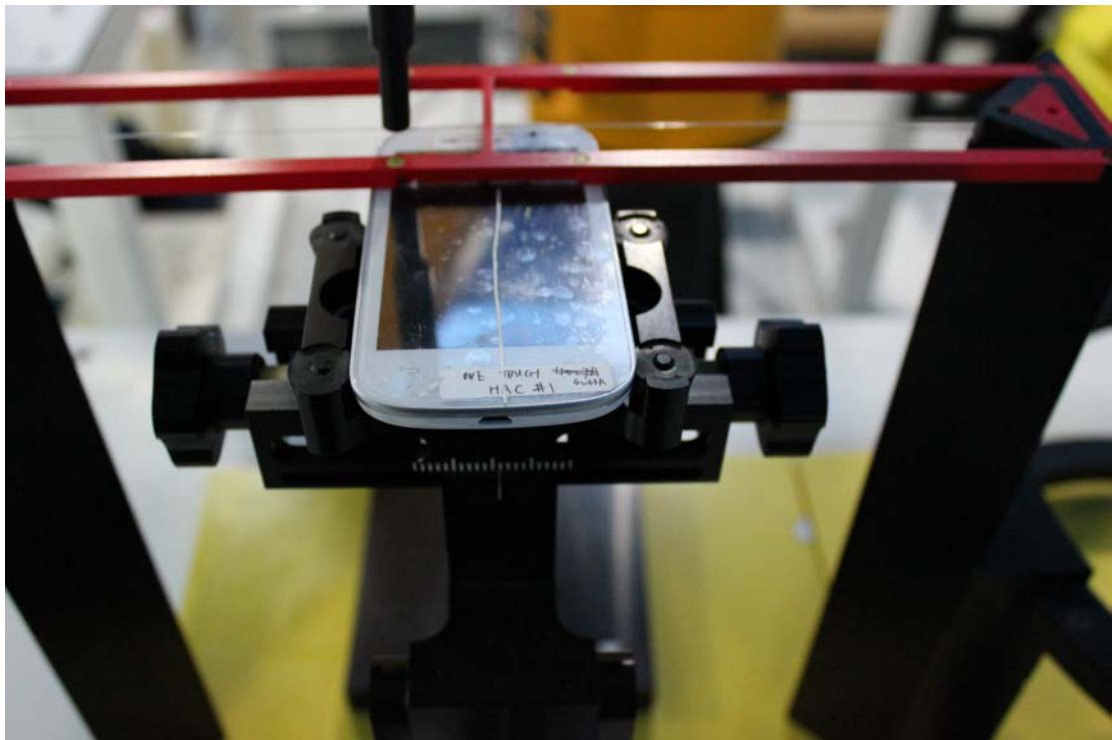
Picture 2: EUT Positioning for RF
