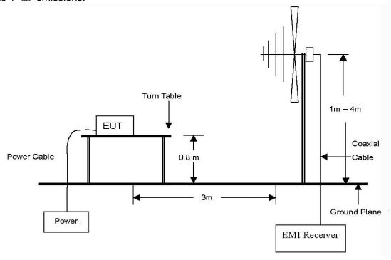
The diagram below shows the test setup that is utilized to make the measurements for emission from 1  $\oplus$  to 40  $\oplus$  emissions.
