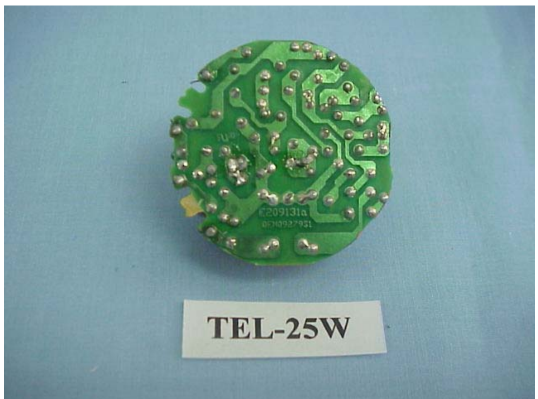
FIGURE 12 ENERGY SAVING LAMP (M/N: TEL-25W) MAIN BOARD (SOLDERED SIDE)
