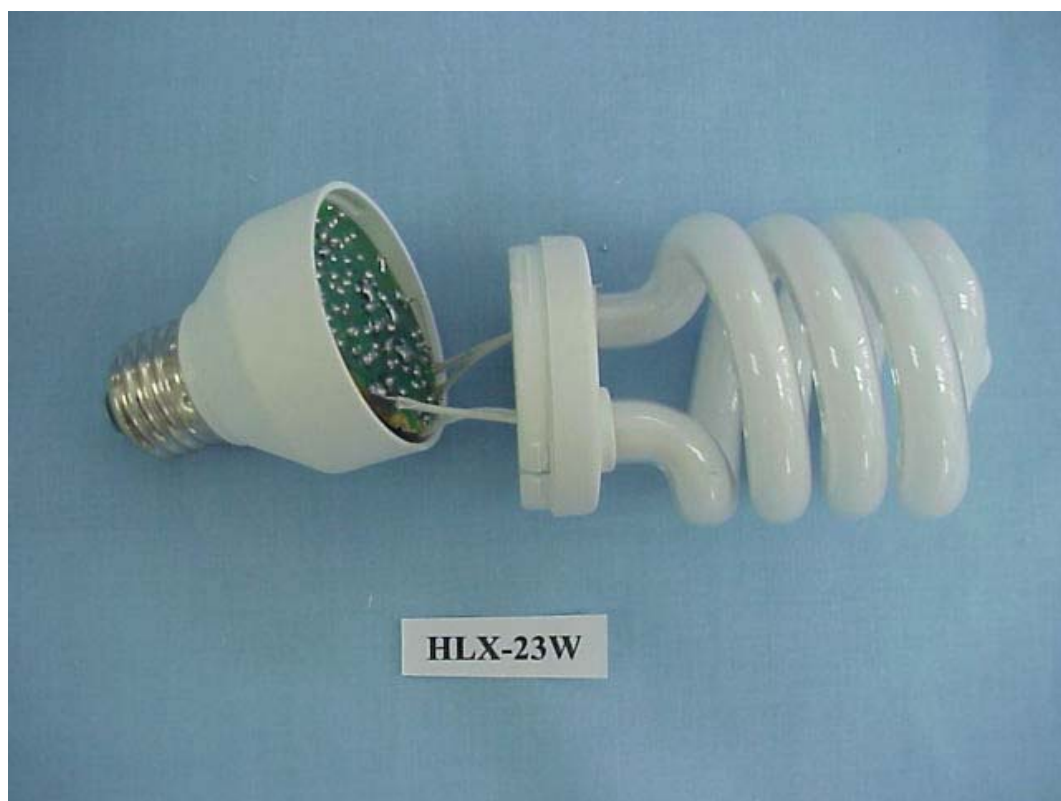
Figure 19 ENERGY SAVING LAMP (M/N: HLX-23W) COVER REMOVED
