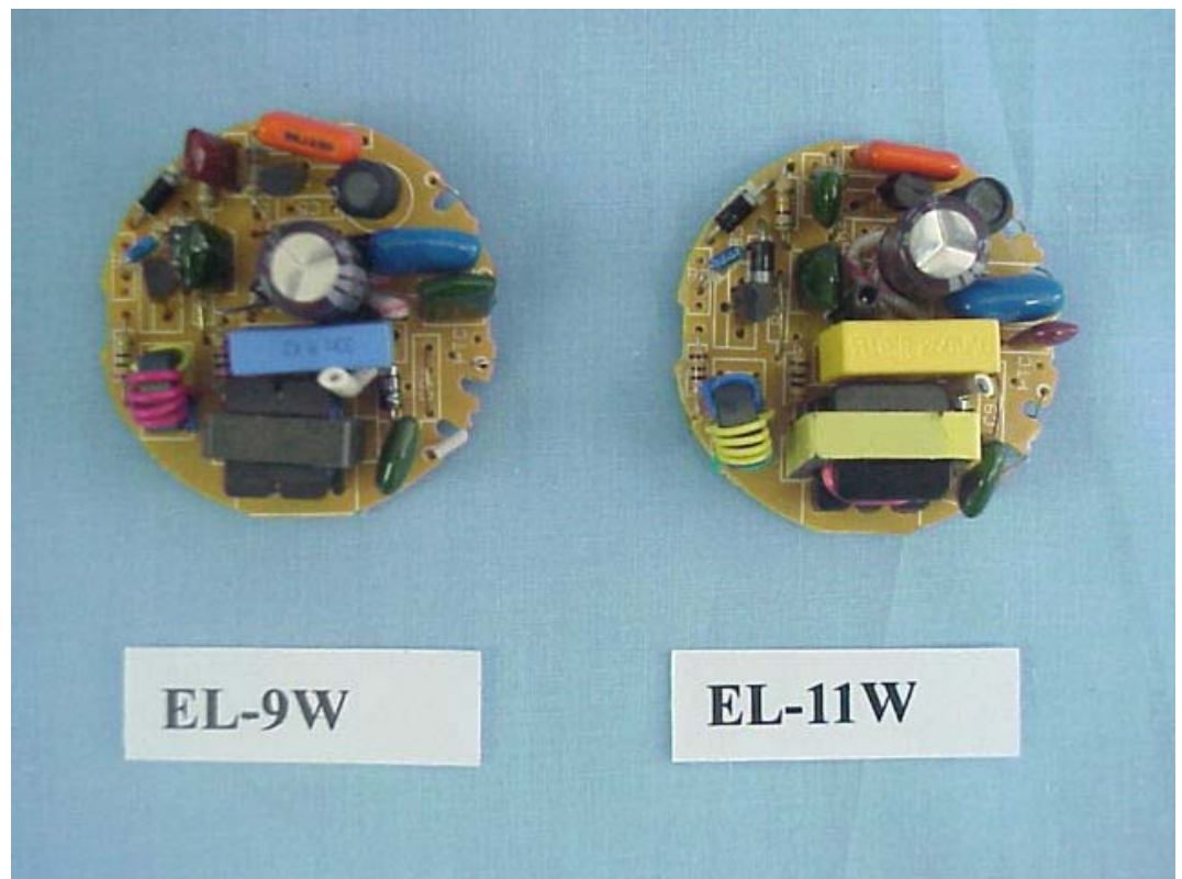
FIGURE 2 ENERGY SAVING LAMP (M/N: EL-9W/11W) MAIN BOARD (COMPONENT SIDE)
