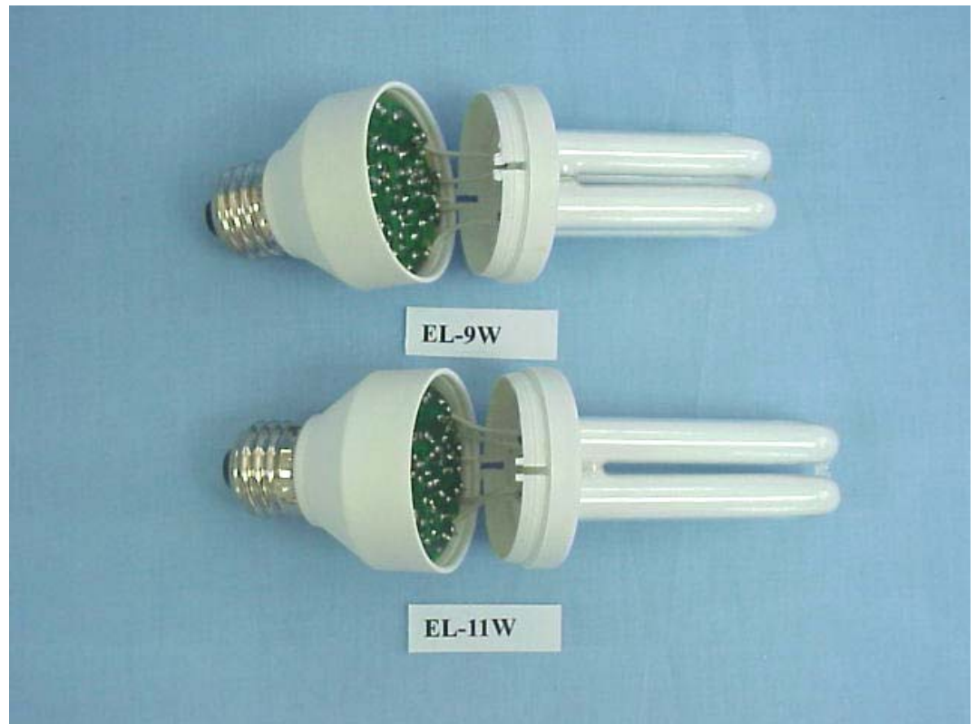
FIGURE 1 ENERGY SAVING LAMP (M/N: EL-9W/11W) COVER REMOVED
