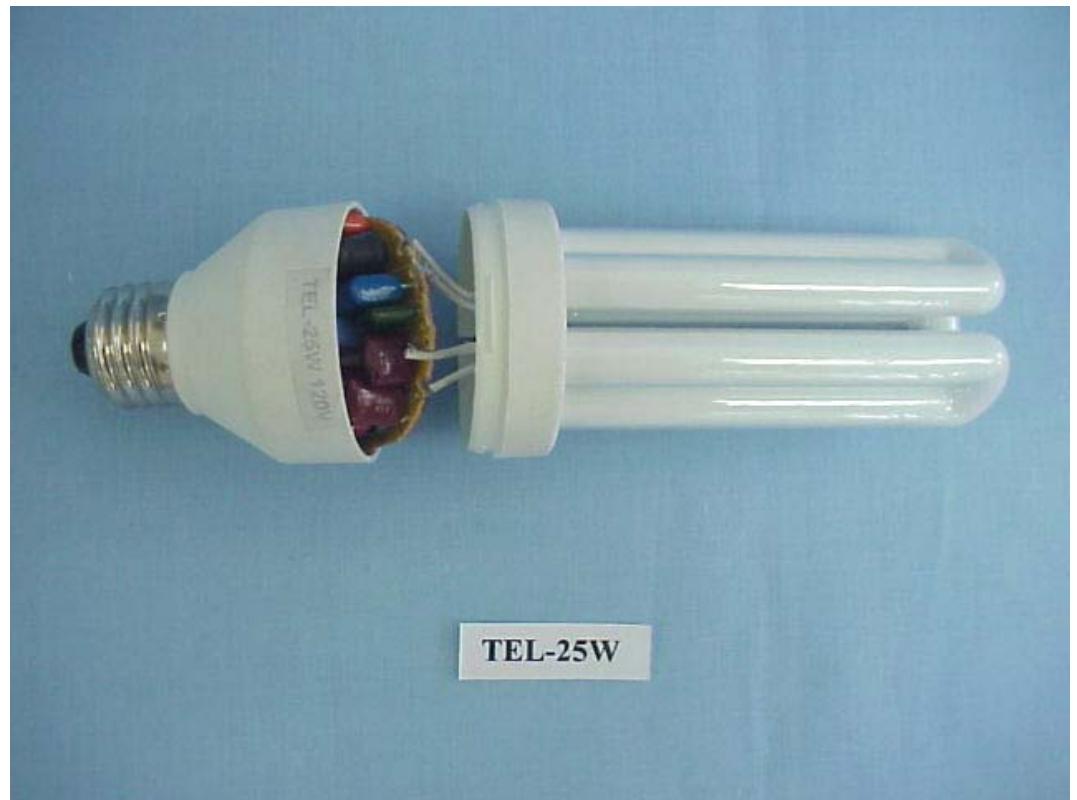
FIGURE 10 ENERGY SAVING LAMP (M/N: TEL-25W) COVER REMOVED
