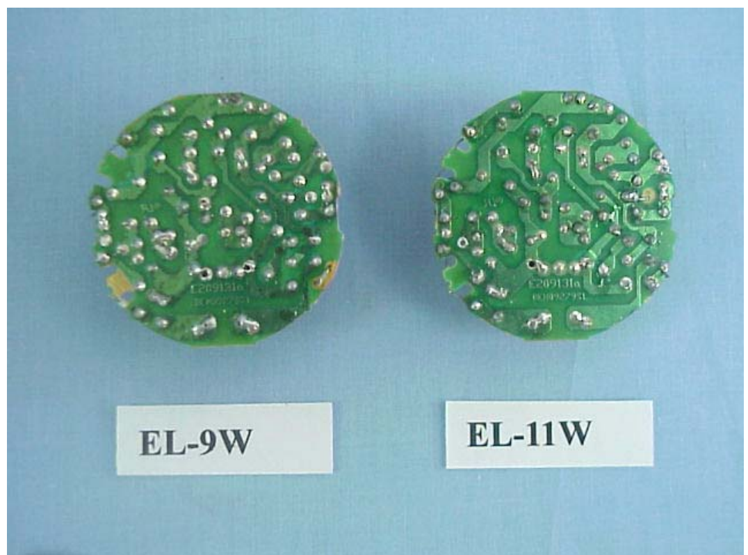
FIGURE 3 ENERGY SAVING LAMP (M/N: EL-9W/11W) MAIN BOARD (SOLDERED SIDE)
