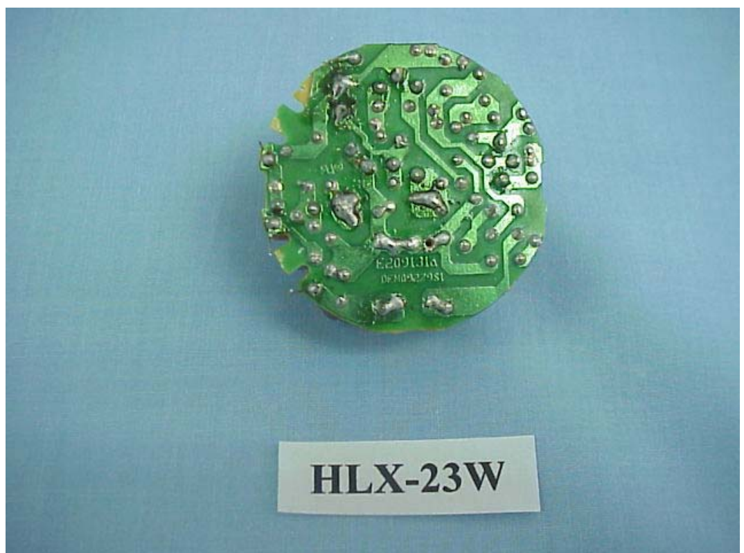
FIGURE 21 ENERGY SAVING LAMP (M/N: HLX-23W) MAIN BOARD (SOLDERED SIDE)
