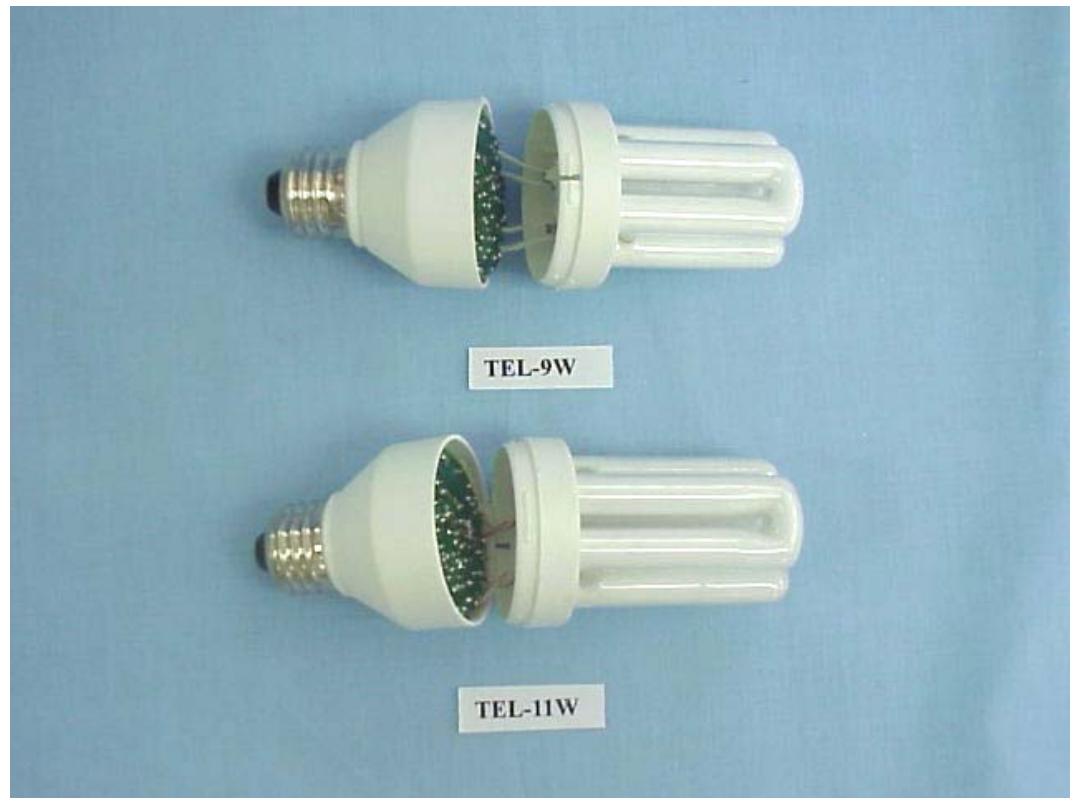
Figure 4 ENERGY SAVING LAMP (M/N: TEL-9W/11W) COVER REMOVED
