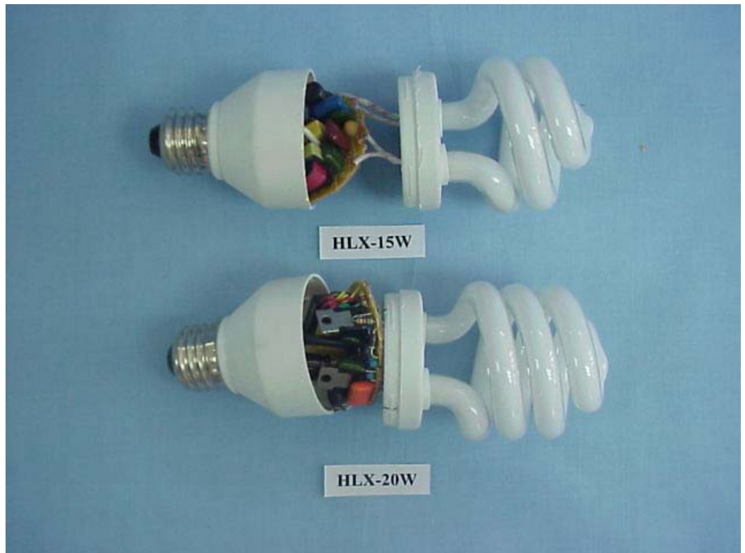
FIGURE 16 ENERGY SAVING LAMP (M/N: HLX-15W/20W) COVER REMOVED
