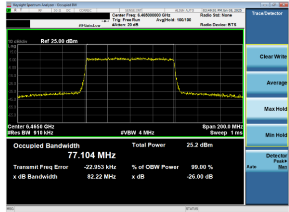
Plot 7-7. 26dB & 99% Bandwidth Plot Antenna 5T (80MHz) 802.11ax (UNII Band 6) – Ch. 103)
