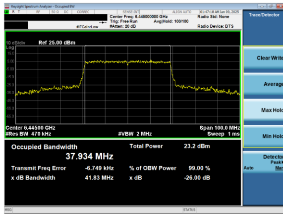
Plot 7-62. 26dB & 99% Bandwidth Plot Antenna 1b (40MHz 802.11ax (UNII Band 6) – Ch. 99)
