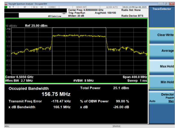
Plot 7-36. 26dB & 99% Bandwidth Plot Antenna 3b (160MHz 802.11ax (UNII Band 6) – Ch. 111)
