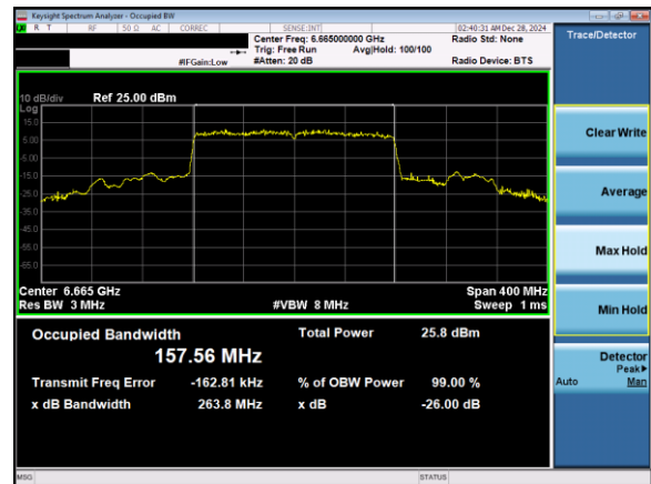
Plot 7-40. 26dB & 99% Bandwidth Plot Antenna 3b (160MHz 802.11ax (UNII Band 7) – Ch. 143)
