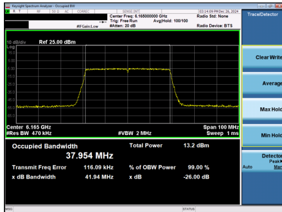
Plot 7-70. 26dB & 99% Bandwidth Plot Antenna 1b (40MHz 802.11ax (UNII Band 5) – Ch. 43)
