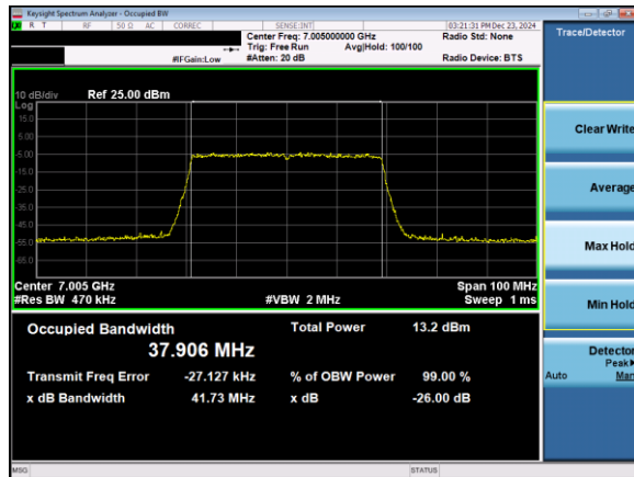
Plot 7-26. 26dB & 99% Bandwidth Plot Antenna 5T (40MHz 802.11ax (UNII Band 8) – Ch. 211)
