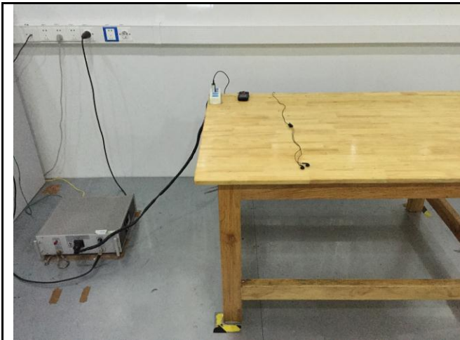
Conducted Emissions Test Setup Front View
