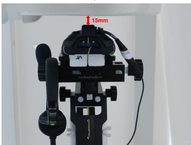
Back with Earphone 2, Test Separation 15 mm
