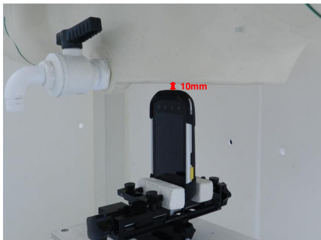
Bottom Side, Test Separation 10 mm
