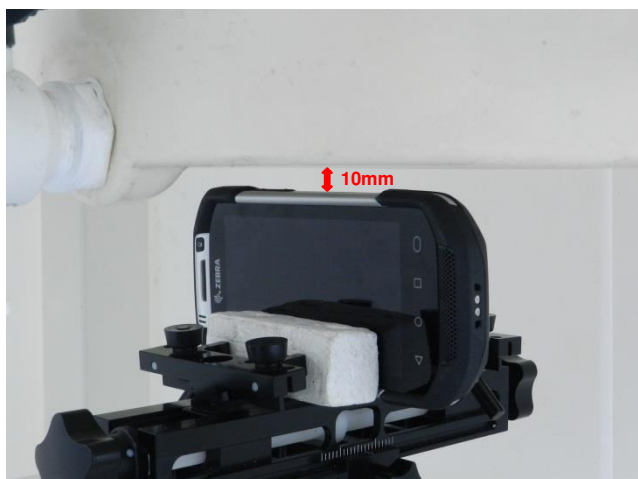
Right Side, Test Separation 10 mm
