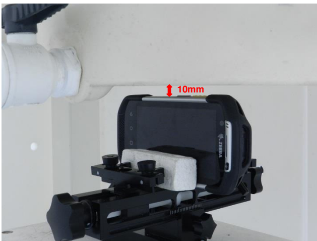
Left Side, Test Separation 10 mm
