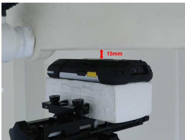
Back, Test Separation 15 mm
