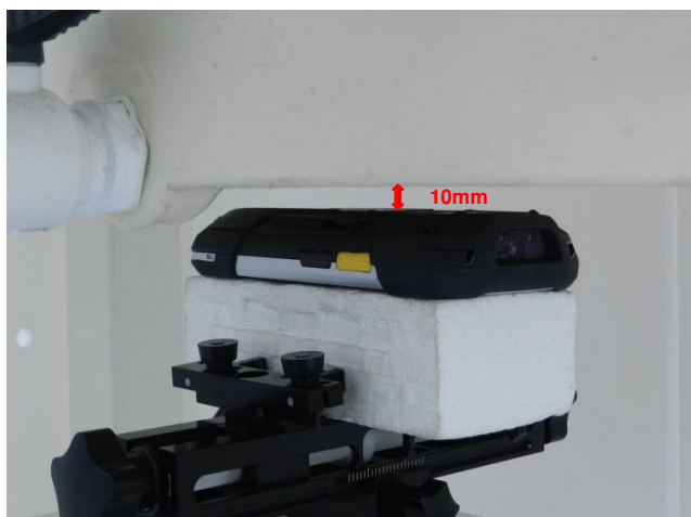
Back, Test Separation 10 mm
