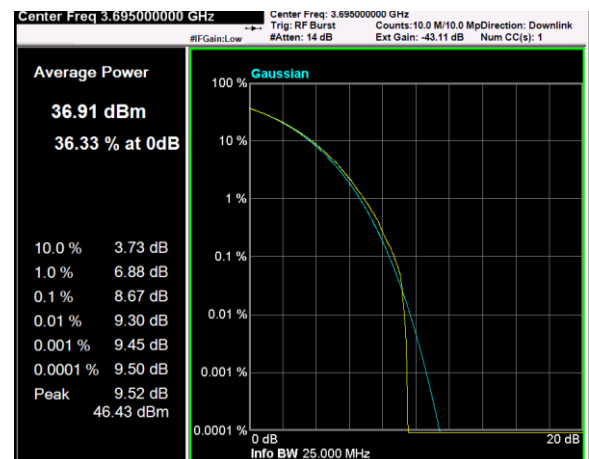
Channel: TOP, Modulation: 16QAM, BW=10MHz, CCDF
