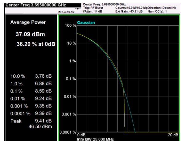
Channel: TOP, Modulation: 256QAM, BW=10MHz, CCDF
