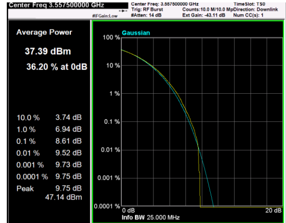
Channel: BOTTOM, Modulation: QPSK, BW=15MHz, CCDF
