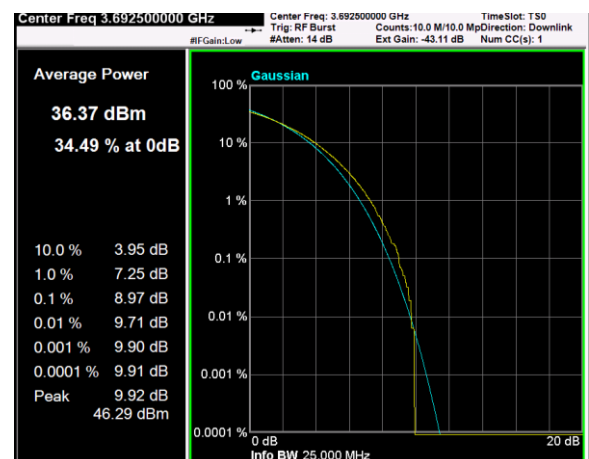
Channel: TOP, Modulation: 256QAM, BW=15MHz, CCDF
