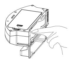
H. Dry the dust box and filter assembly, and keep it dry to ensure its service life.
