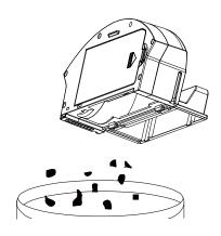
E. Take out the two filter screens: the high-efficiency screen and the primary-efficiency screen. It is not recommended to wash high-efficiency screen with water. Tap gently to remove dust.
