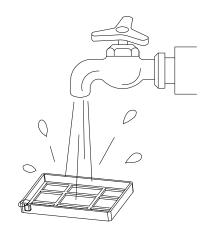
G. The dust box is scrubbed clean with dishcloth. Do not allow water to seep into the fan port when cleaning.
