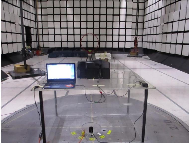
**Photograph 5. Field Strength Below 30 MHz, Test Setup Rear View**
