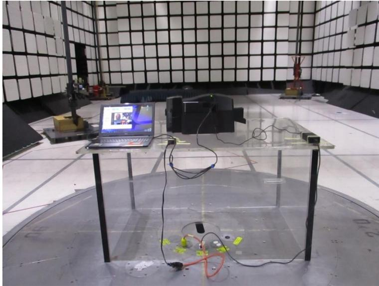
**Photograph 7. Field Strength Above 30 MHz, Test Setup Rear View**
