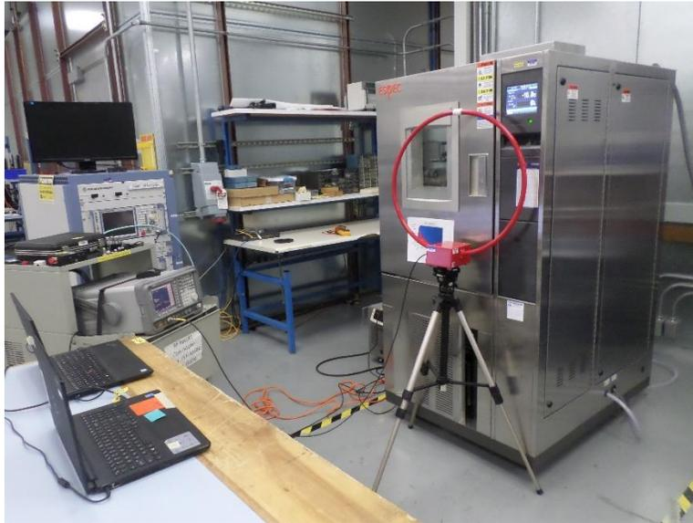
**Photograph 9. Frequency Stability Test Setup**
