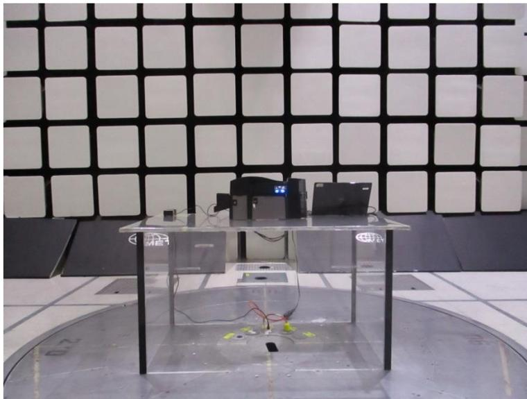
**Photograph 6. Field Strength Above 30 MHz, Test Setup Front View**
