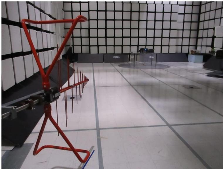
**Photograph 8. Field Strength Above 30 MHz, Test Setup Antenna View**
