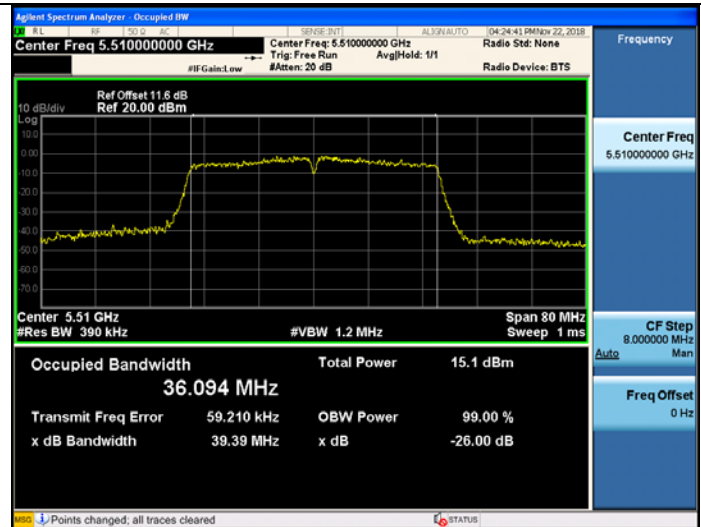
802.11ac(VHT40) UNII 2C BAND 26dB Bandwidth(CH 102)
