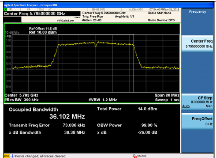
802.11n_HT40 UNII 3 BAND 26dB Bandwidth (CH 159)
