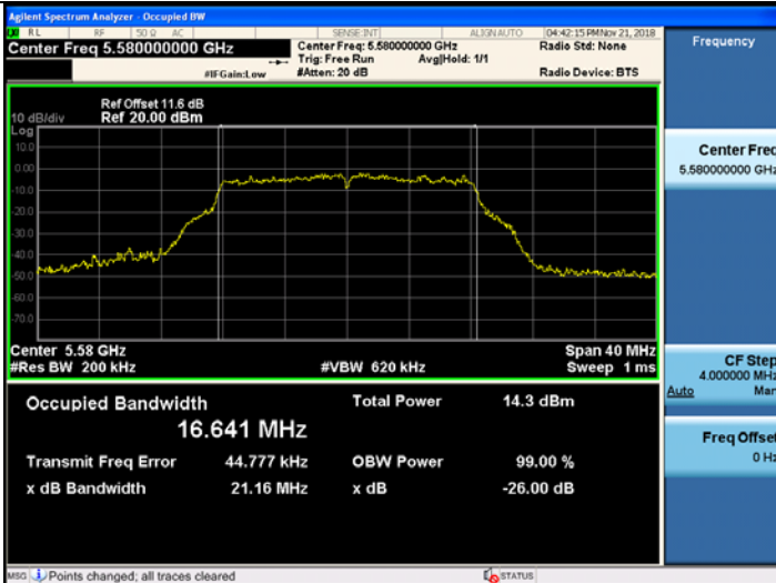
802.11a UNII 2C BAND 26dB Bandwidth (CH116)
