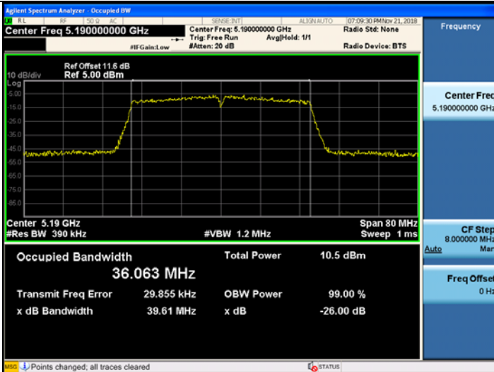
802.11n_HT40 UNII 2C BAND 26dB Bandwidth(CH 110)
