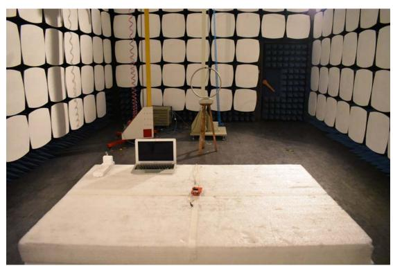
3. Radiated emission (9KHz-30MHz)
