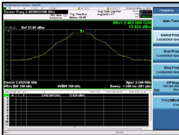
GFSK LOW CHANNEL, CARRIER LEVEL
