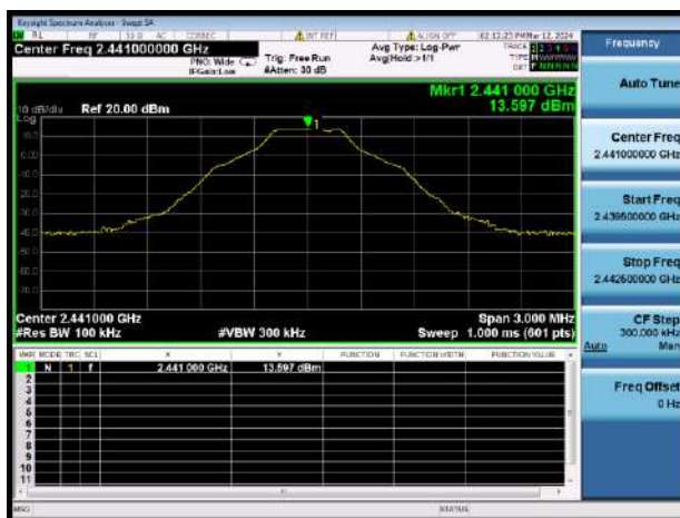
GFSK MIDDLE CHANNEL, CARRIER LEVEL
