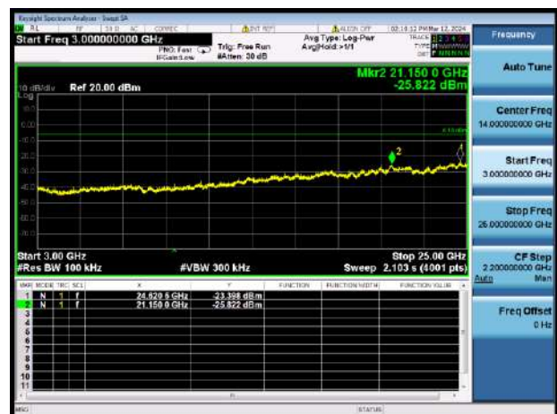
GFSK LOW CHANNEL, SPURIOUS 3 GHz ~ 25 GHz
