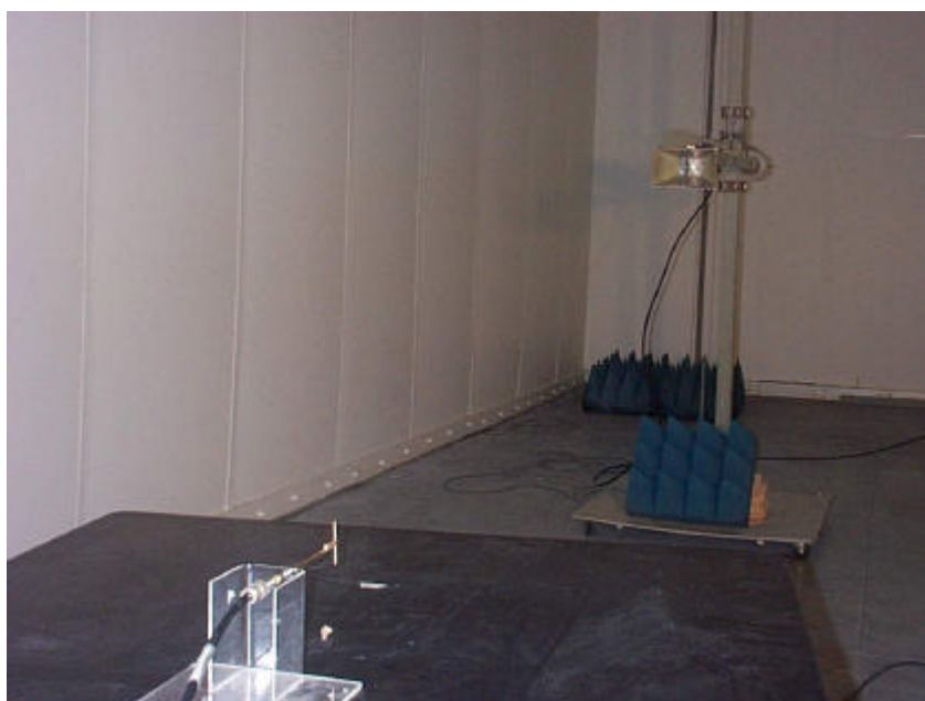
Spurious Emission Measurements Substitution Method, 2.7 GHz Ref. Dipole
