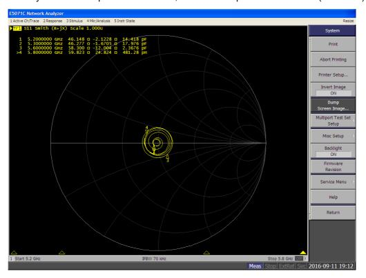
5200MHz Body calibrated return loss: -24.413 dB; Measured return loss: -20.805dB (within 20%) 5300MHz Body calibrated return loss: -25.153 dB; Measured return loss: -25.115dB (within 20%) 5600MHz Body calibrated return loss: -22.766 dB; Measured return loss: -19.000dB (within 20%) 5800MHz Body calibrated return loss: -20.937 dB; Measured return loss: -18.809dB (within 20%)
