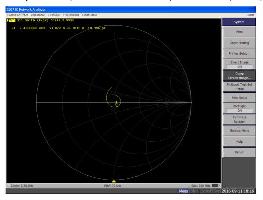
2450MHz Body calibrated return loss: -26.642 dB; Measured return loss: -26.245dB (within 20%)
