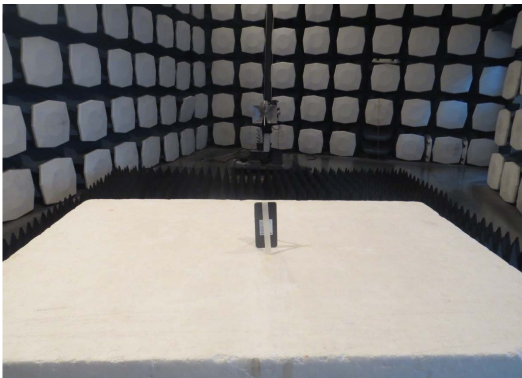
Picture 1: Radiated Spurious Emissions Test setup
