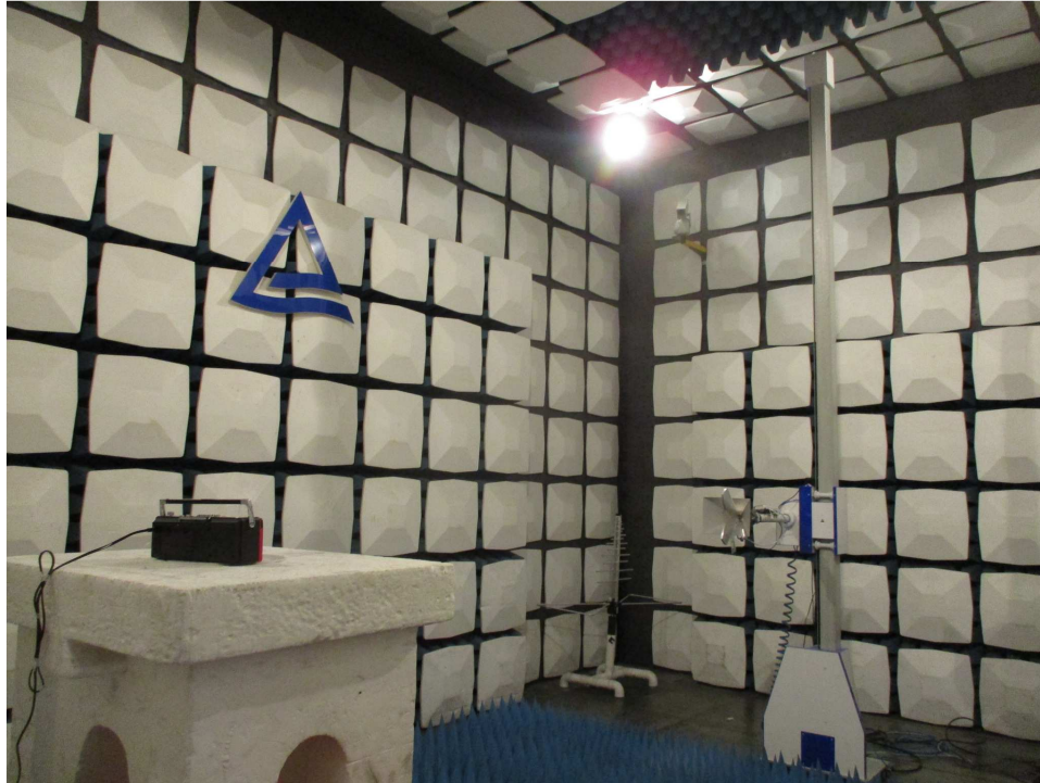
Photograph 4: Set-up for Radiated Spurious Emission, 18GHz - 26.5GHz
