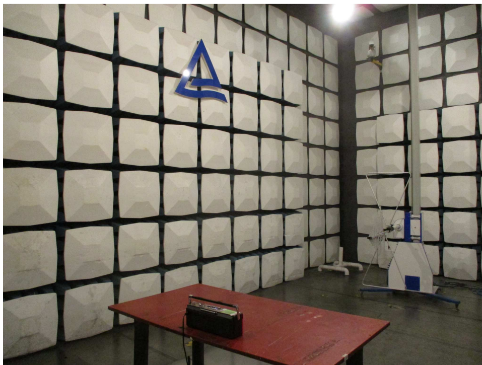
Photograph 2: Set-up for Radiated Spurious Emission, 30MHz - 1GHz
