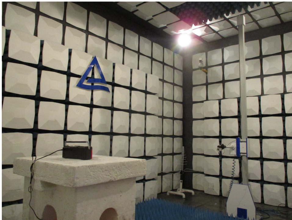
Photograph 4: Set-up for Radiated Spurious Emission, 18GHz - 26.5GHz
