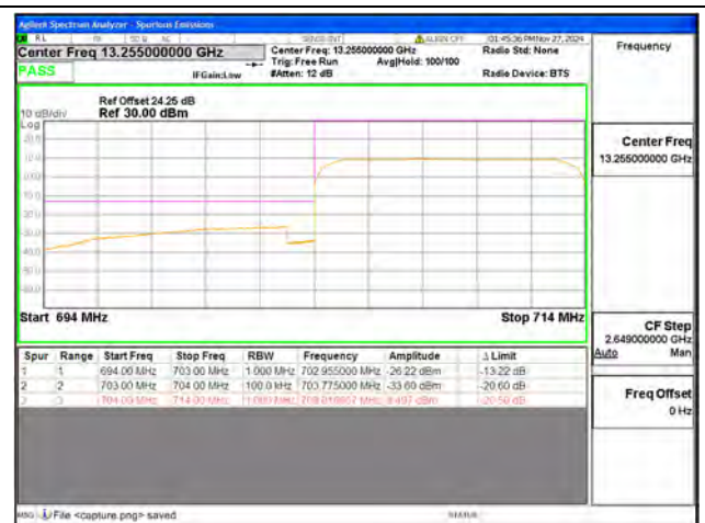
B17 / 10MHz / Low CH / QPSK / FULL RB
