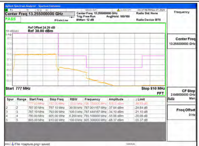
B13 / 10MHz / High CH / QPSK / FULL RB
