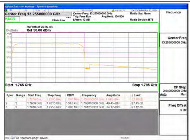
B66 / 15MHz / High CH / QPSK / FULL RB
