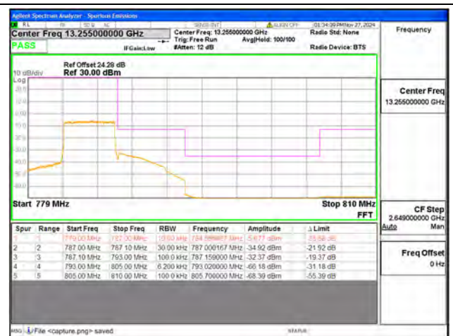
B13 / 5MHz / High CH / QPSK / FULL RB
