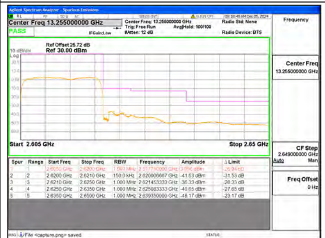
B38 / 15MHz / High CH / QPSK / FULL RB
