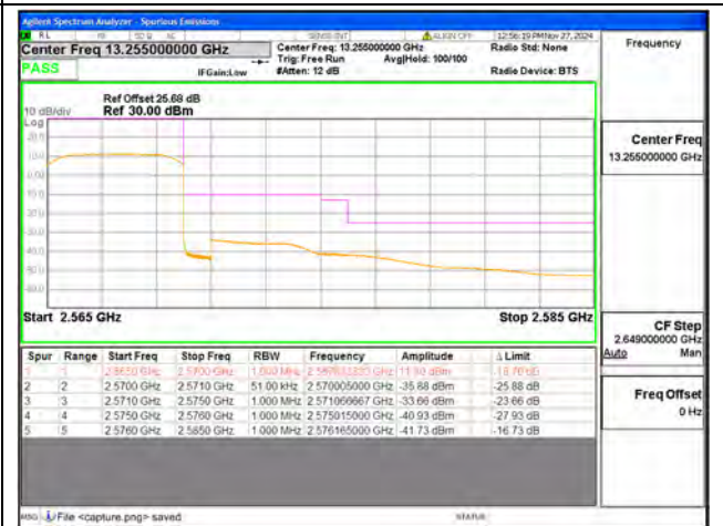
B7 / 5MHz / High CH / QPSK / FULL RB
