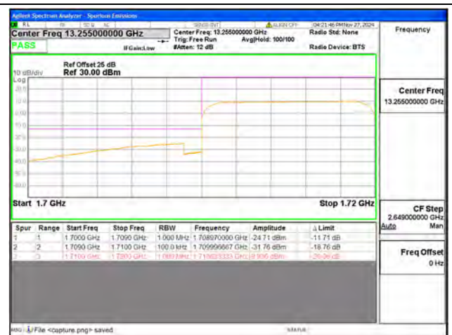
B66 / 10MHz / Low CH / QPSK / FULL RB
