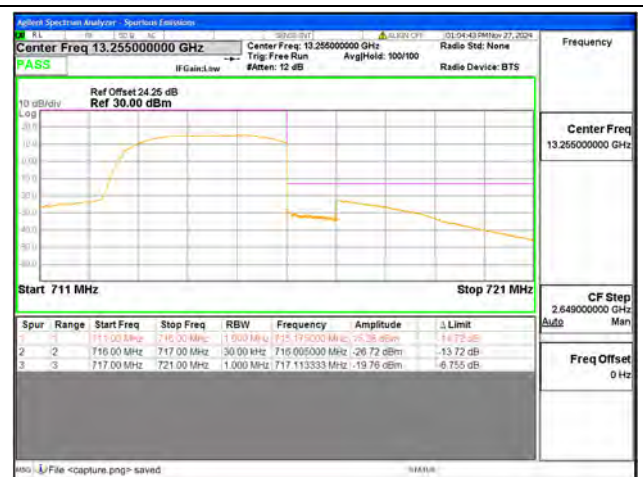
B12 / 3MHz / High CH / QPSK / FULL RB
