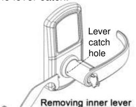
insert tool into lever catchholt & push back the lever catch, remove lever.
