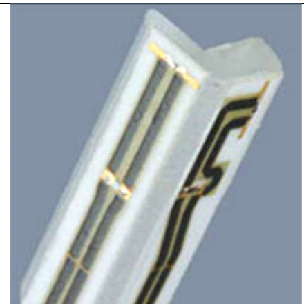
Photo of E-field Probe
