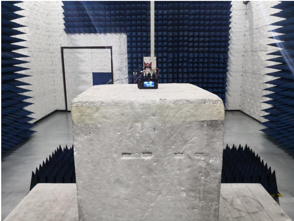
RADIATED EMISSION TEST SETUP ABOVE 1GHz
