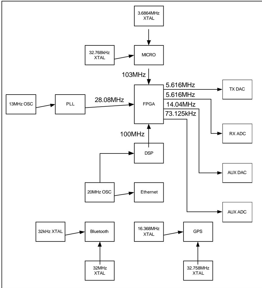
**Figure 2. Clock Diagram**
