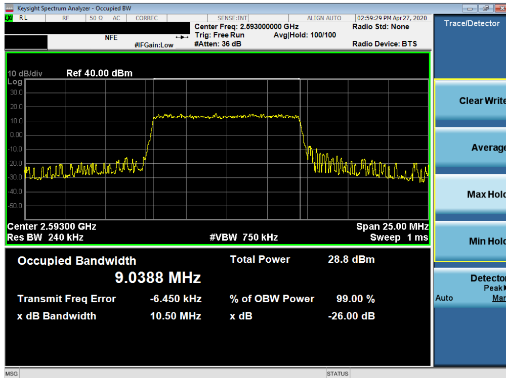
Plot 7-21. Occupied Bandwidth Plot (LTE Band 41(PC3) - 10MHz 64-QAM - Full RB Configuration)
