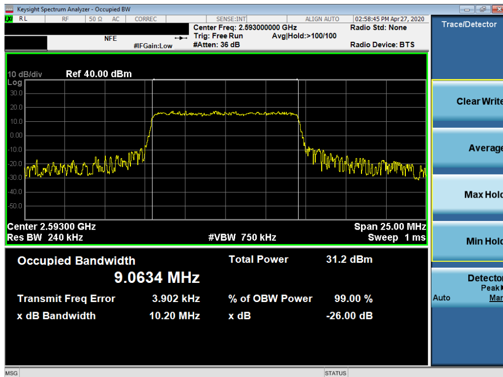
Plot 7-19. Occupied Bandwidth Plot (LTE Band 41(PC3) - 10MHz QPSK - Full RB Configuration)
