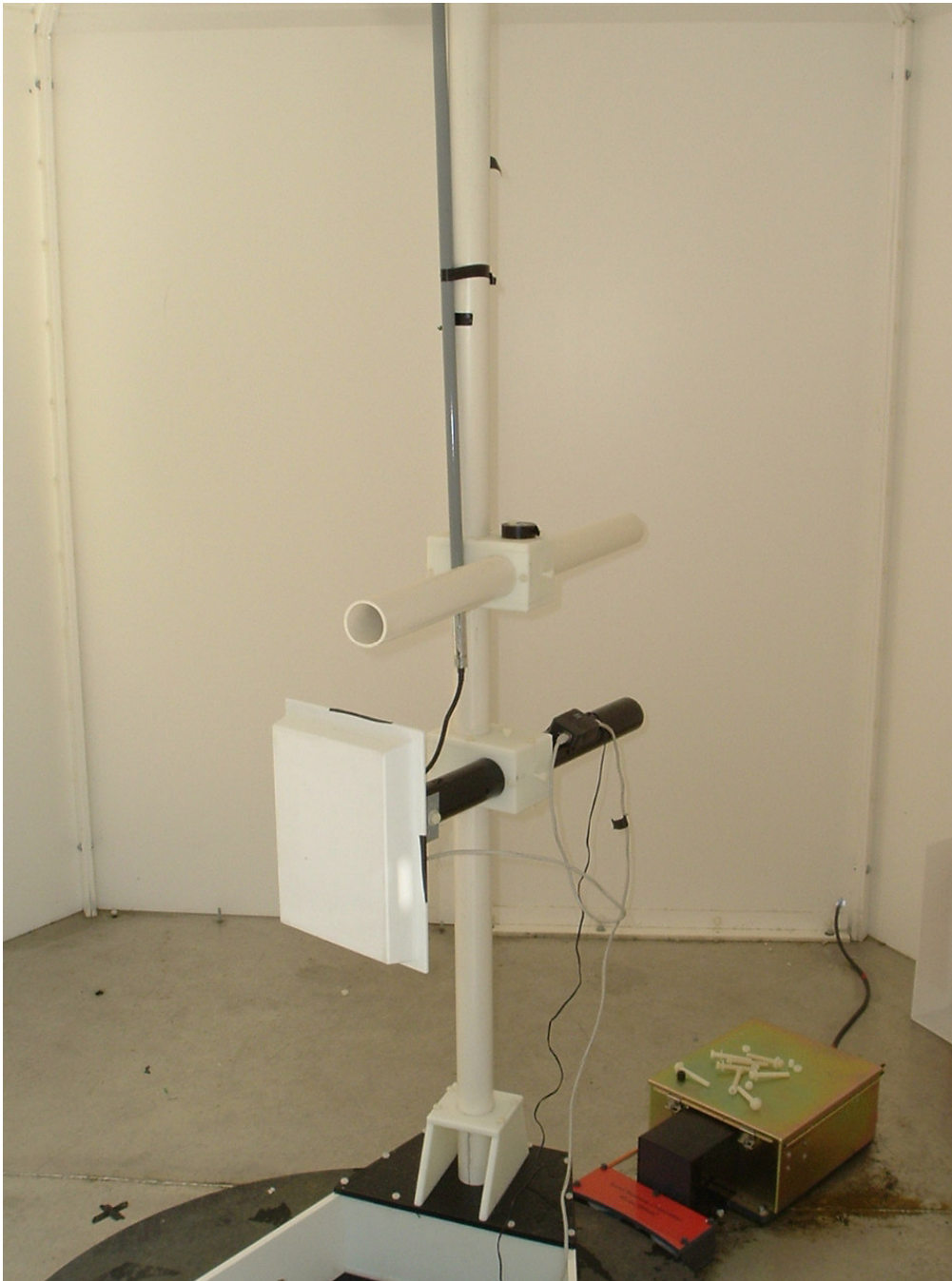
Radiated Emissions Test Setup – 12 dBi Dipole
