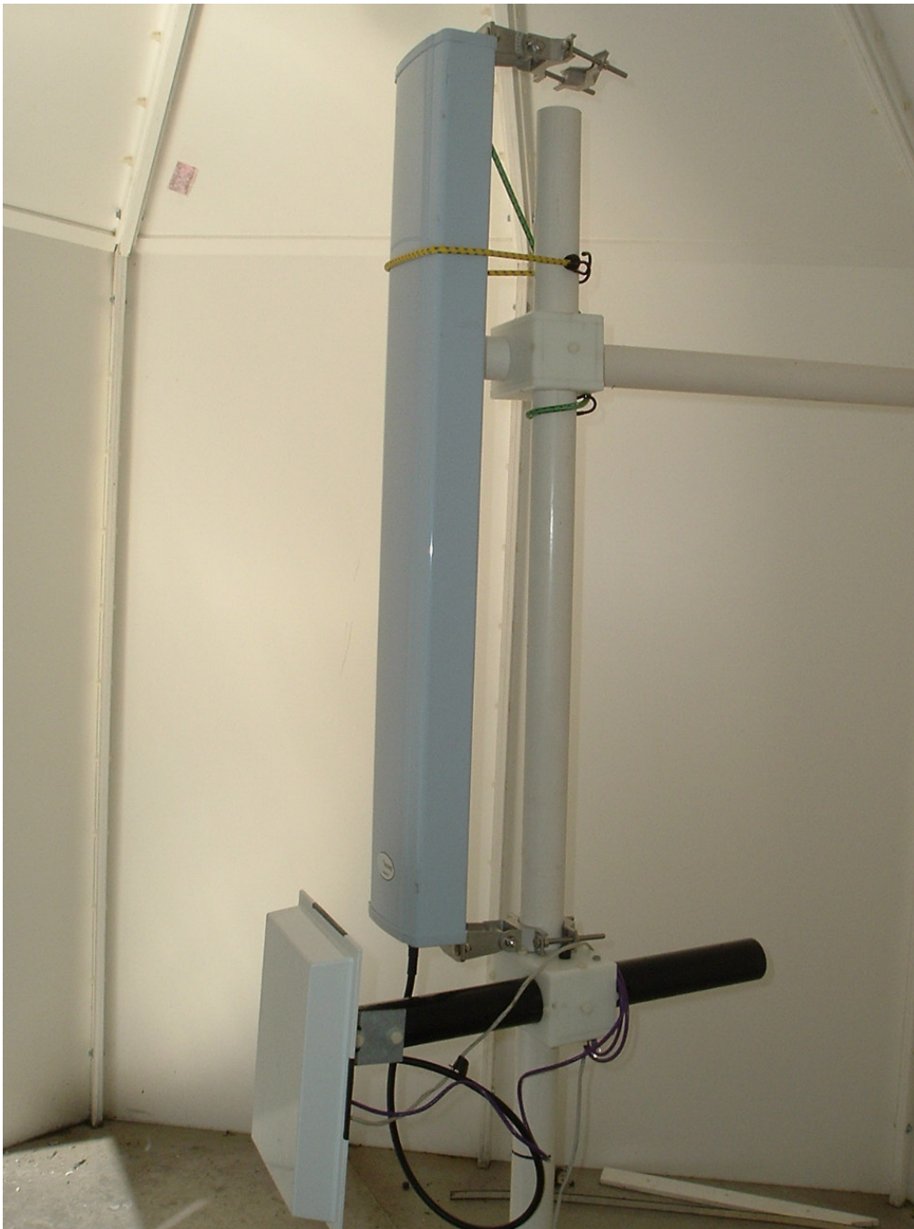
Radiated Emissions Test Setup – 17 dBi Sector
