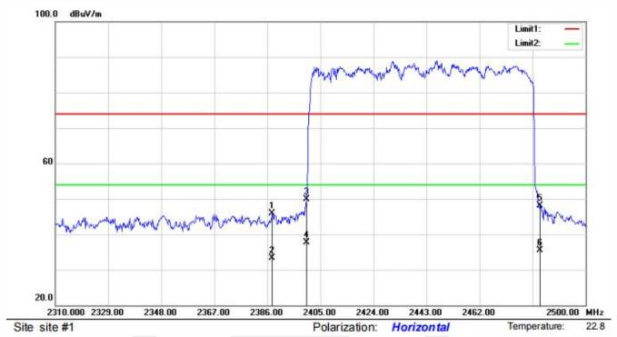
Test Model Spurious Emission in Restricted Band 2310-2390MHz and 2400-2483.5MHz
