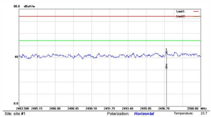
Test Model Spurious Emission in Restricted Band 2483.5-2500MHz
