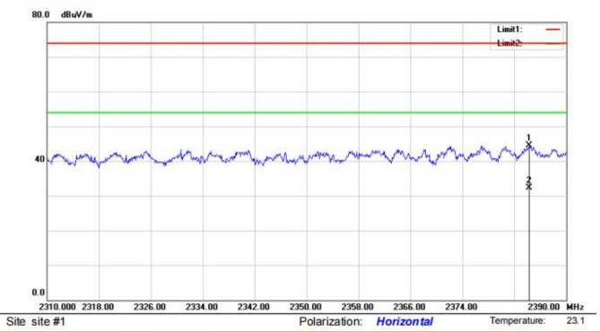
Test Model Spurious Emission in Restricted Band 2310-2390MHz
