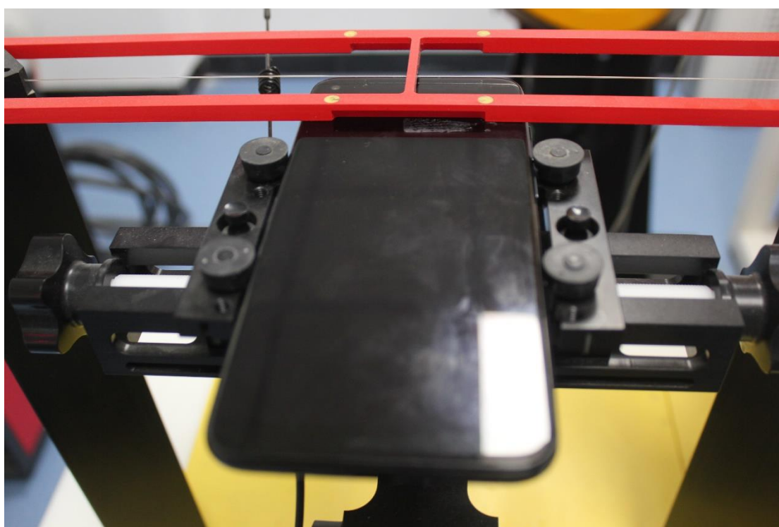
Picture 2: EUT Positioning for RF/T-coil
