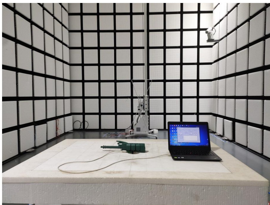
Fig. 2 Radiated emission setup photo(30MHz-1GHz)
