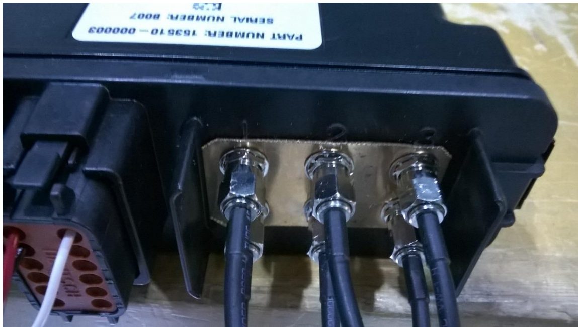
Figure 1 – Modifications done after testing (copper plate installed)
