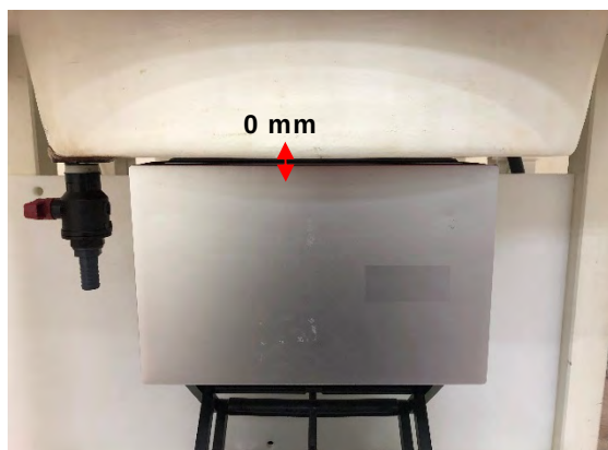
Fig.3 EUT Bottom side to flat phantom
