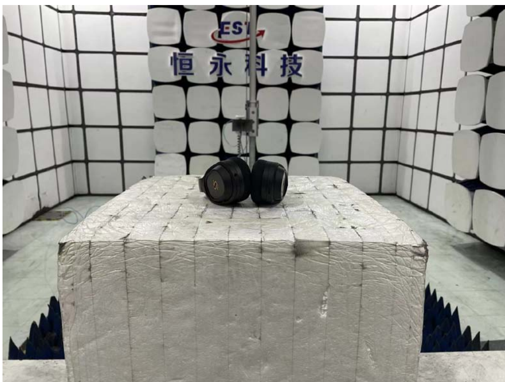
Radiated emission test: Above 1GHz
