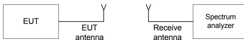
Figure 7.7.1 Band edge emission test setup
