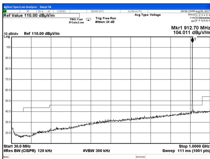
Plot 7.6.10 Radiated emission measurements from 30 to 1000 MHz at the mid carrier frequency
