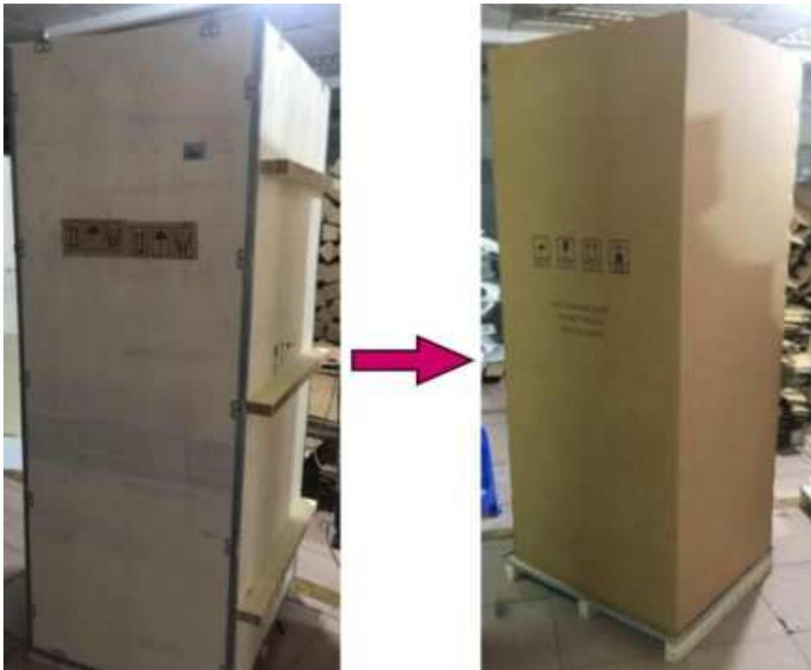
Inside the wooden crate, the kiosk in the cardboard shield can be found. This cardboard shield can be slid out from the top of the kiosk.
