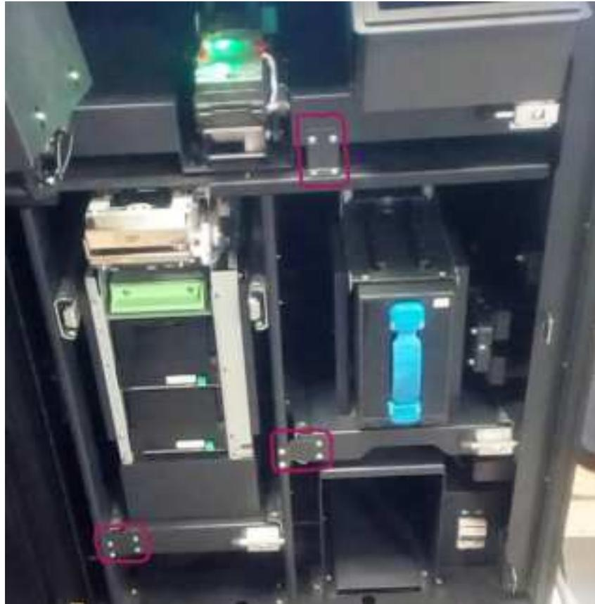
3. Remove the stoppers to allow the smooth operation of the sliders.
