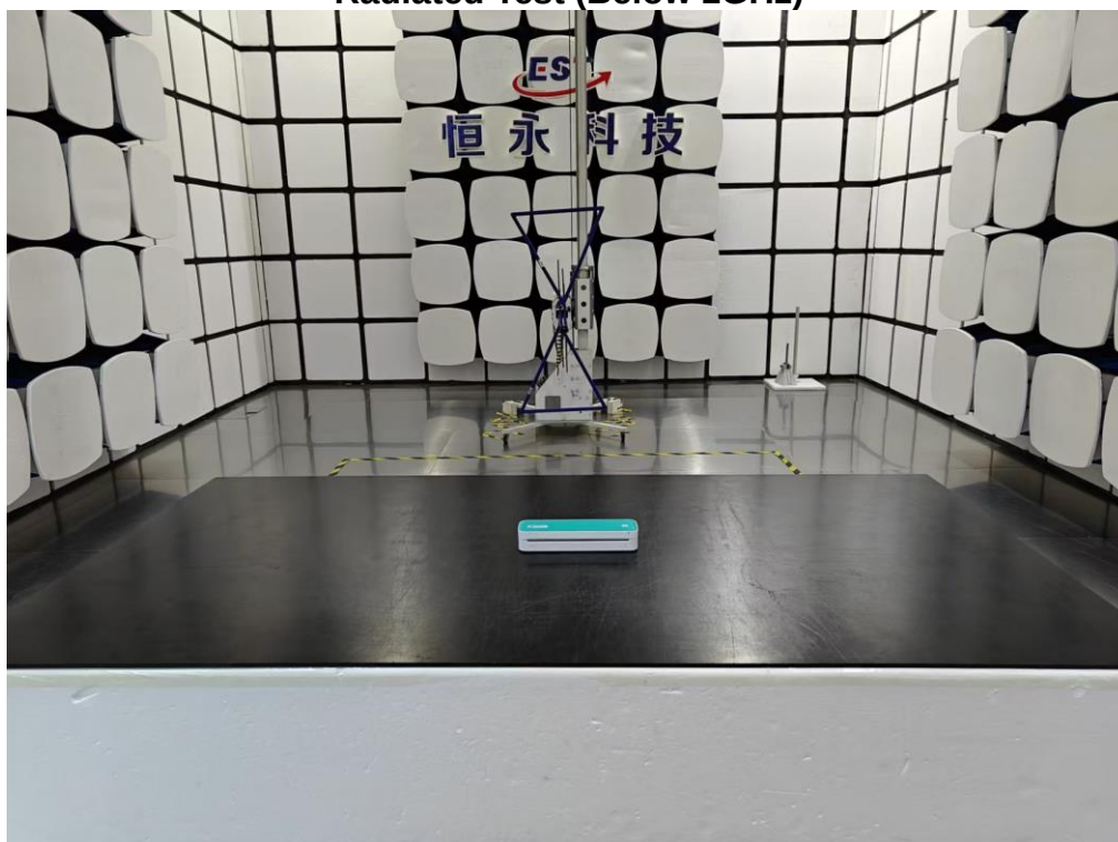
Radiated Test (Below 1GHz)
