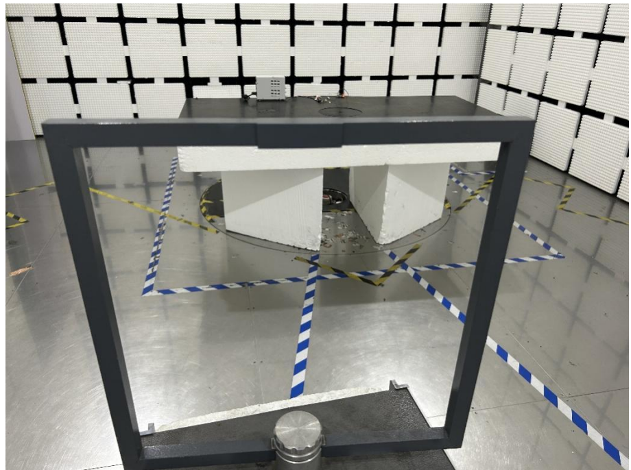
Radiation Emission Test Setup (Below 30MHz)
