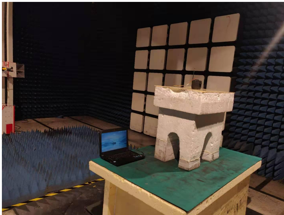
Spurious Emission Test Setup (Above 1GHz)
