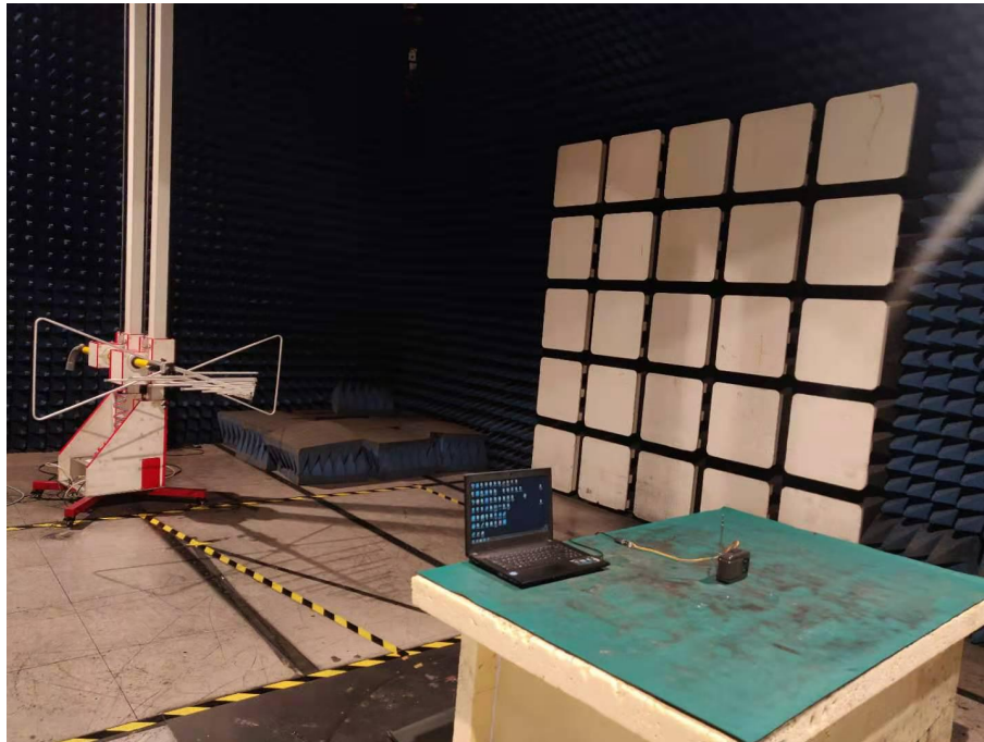
Spurious Emission Test Setup (Below 1GHz)
